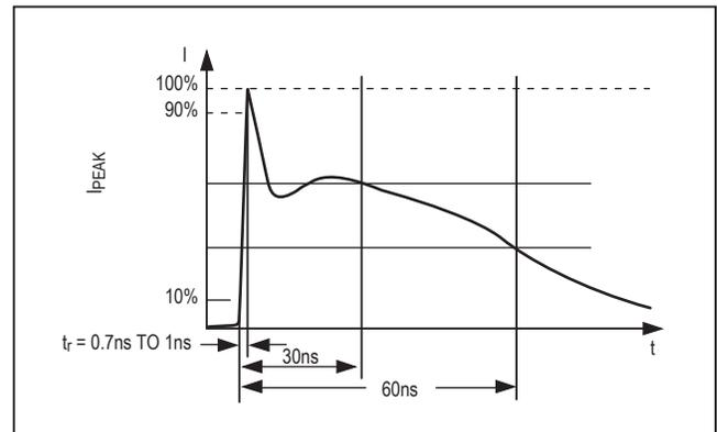
Figure 10d. IEC 1000-4-2 ESD Generator Current Waveform
