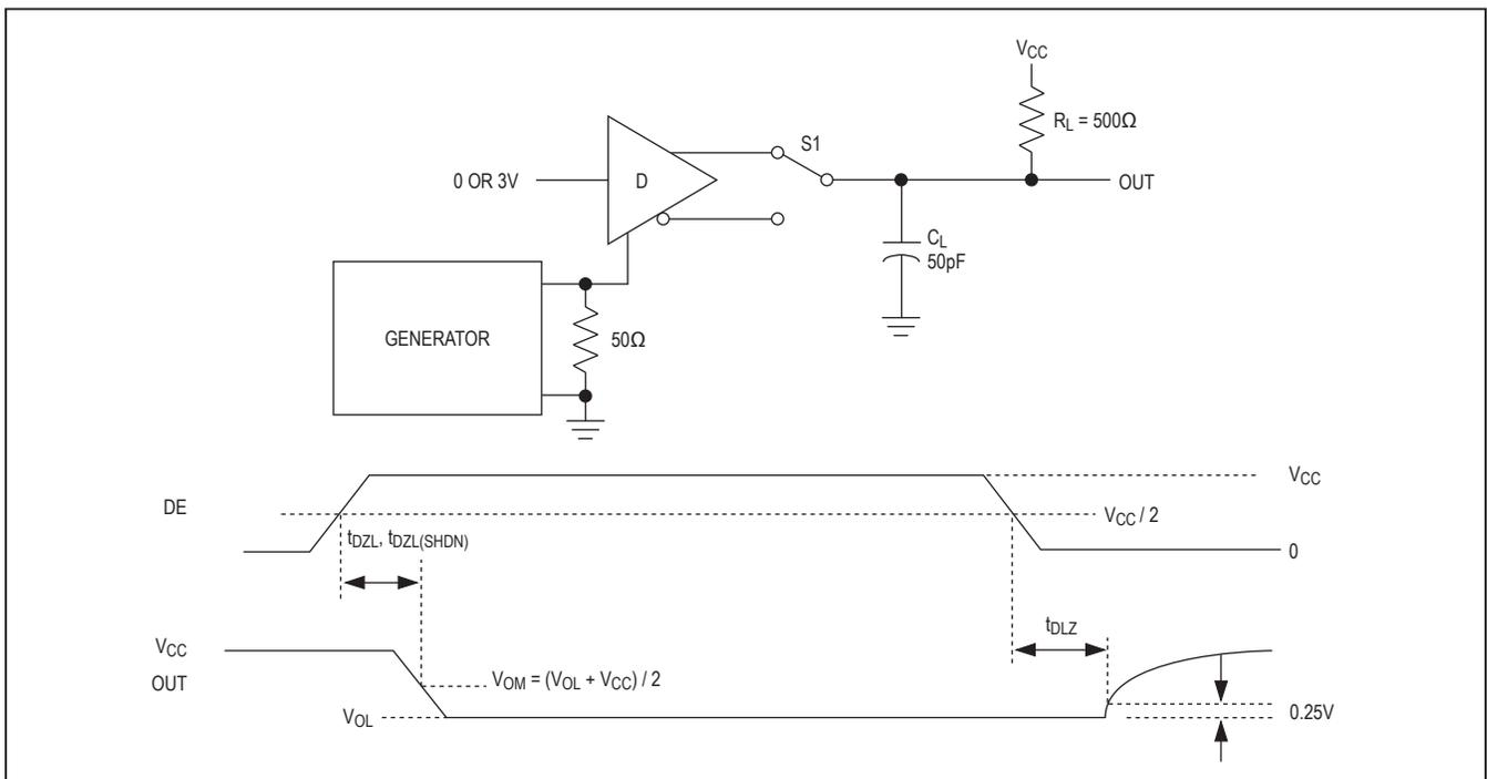
Figure 5. Driver Enable and Disable Times (t<sub>DHZ</sub>, t<sub>DZH</sub>, t<sub>DZH(SHDN)</sub>)
