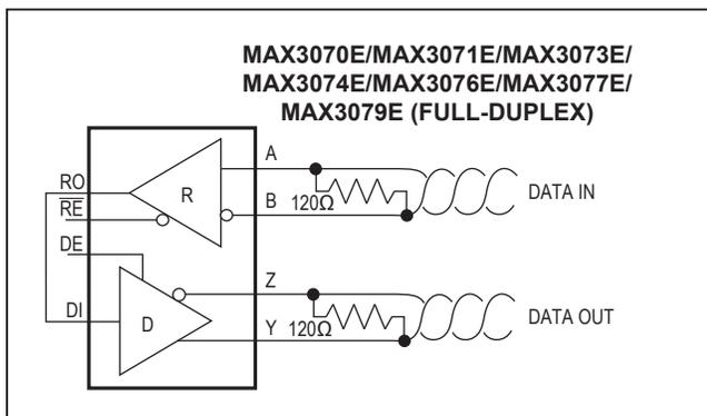
Figure 11. Line Repeater for MAX3070E/MAX3071E/MAX3073E/MAX3074E/MAX3076E/MAX3077E/MAX3079E in Full-Duplex Mode
