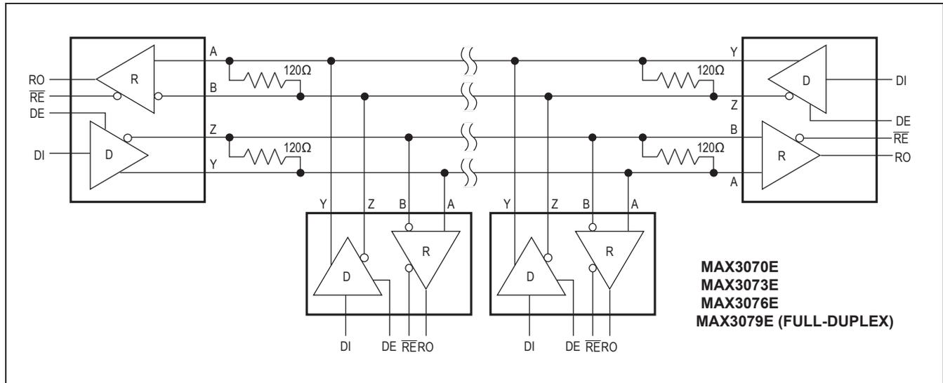
Figure 13. Typical Full-Duplex RS-485 Network
