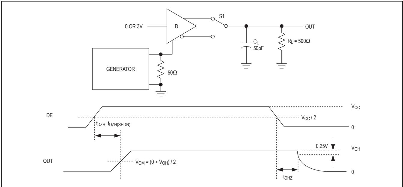
Figure 4. Driver Enable and Disable Times (t<sub>DHZ</sub>, t<sub>DZH</sub>, t<sub>DZH(SHDN)</sub>)
