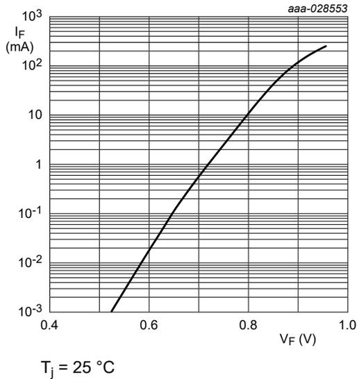
Fig. 5. Forward current as a function of forward voltage; typical values (BZT52H-A/B/C7V5)
