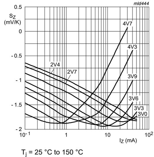
Fig. 6. Temperature coefficient as a function of working current; typical values (BZT52H-A/B/C2V4 to BZT52H-A/B/C4V7)
